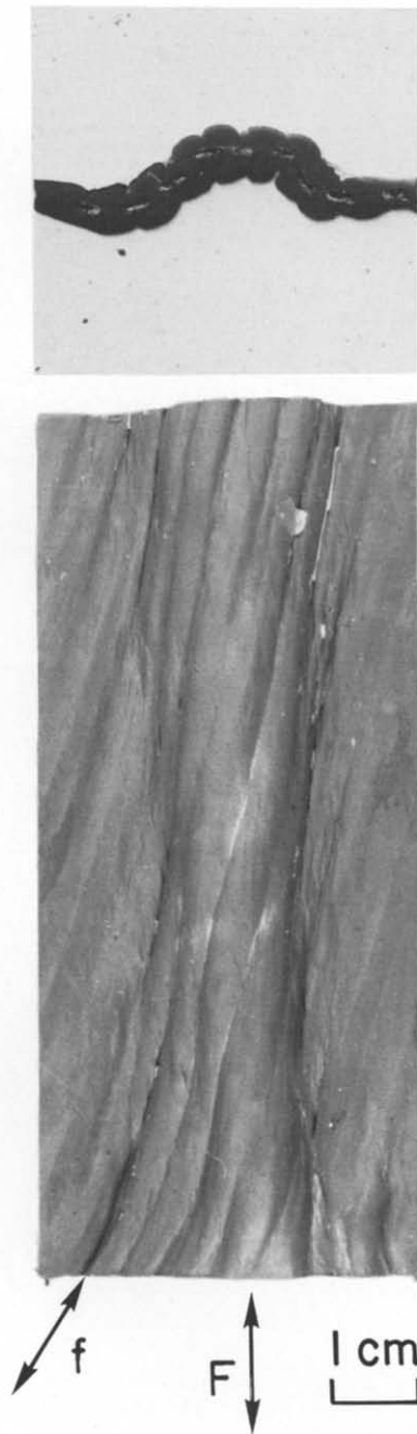
Fig. 3. Plan and profile view of a layer containing linear rods ( f ) at an angle to the major fold axis ( F ). The minor folds form parallel to the rods and contemporaneously with the major fold, but are oblique to the major fold axis F .
